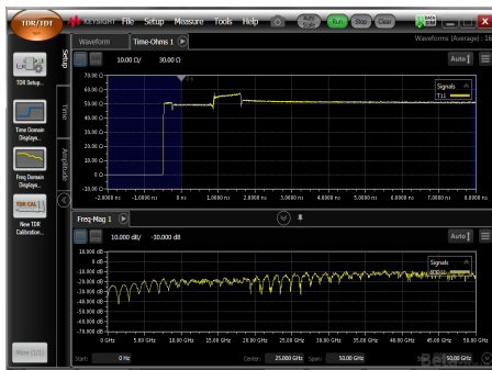
TDR/TDT mode shows the properties (in time/distance or the frequency domain) of electrical channels
